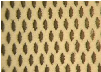
Mesh-supported sorbent (PCI patented design) w. high capacity
